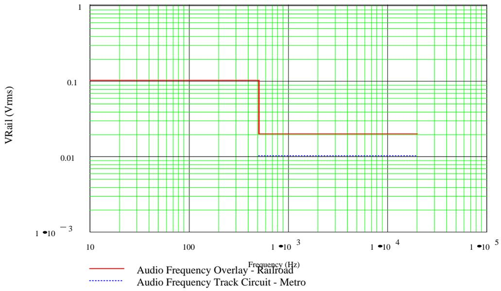
Figure 3: Maximum Allowable Rail-to-Rail Voltage, Under Vehicle
