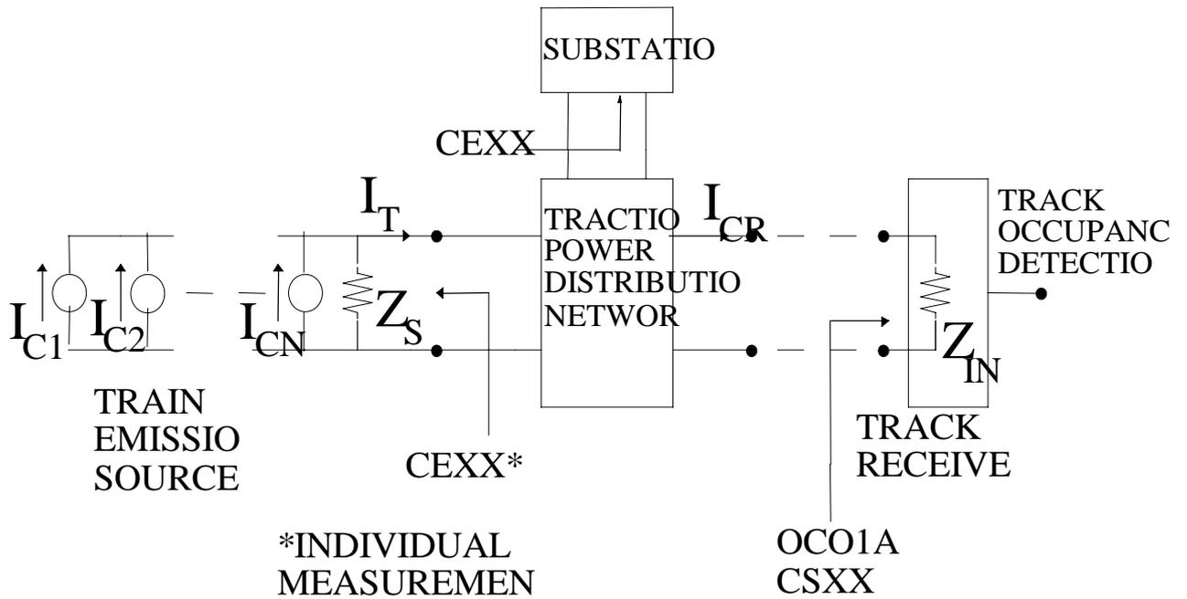
Figure 2: Conducted Interference Equivalent Network
