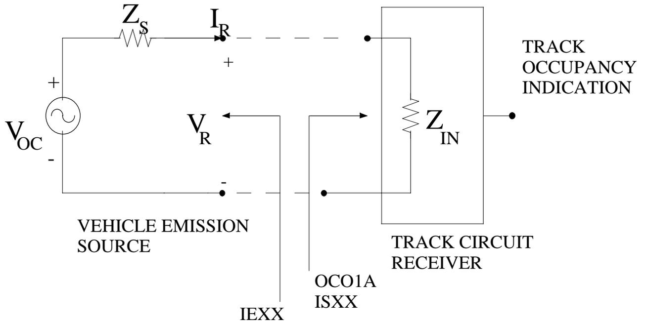
Figure 1: Inductive Interference Circuit
