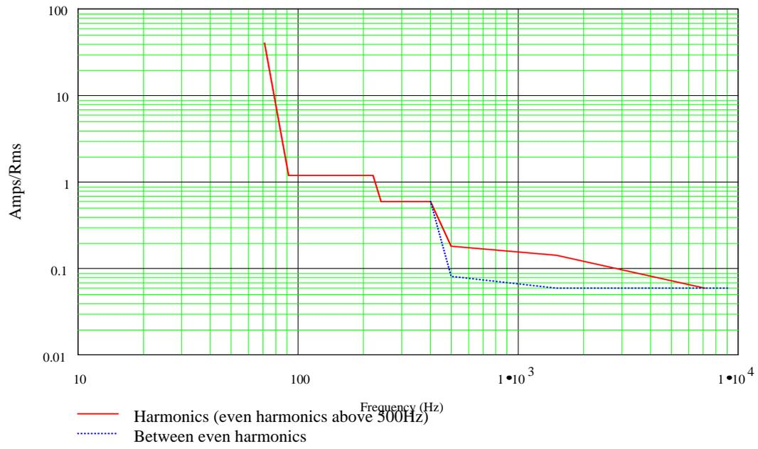
Figure 5: AC Catenary Conducted Emissions Harmonic Current Limit (Train Consist)
