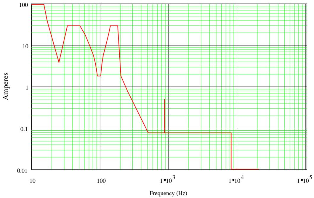
Figure 4: Maximum Allowable Harmonic Emission Current At Line Supply Input (Train Consist)
